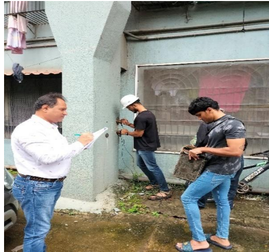
Ultrasonic Pulse Velocity Test (UPV)
