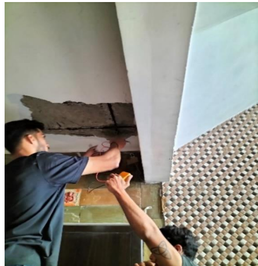
Half Cell Potentiometer Test (Corrosion Test)
