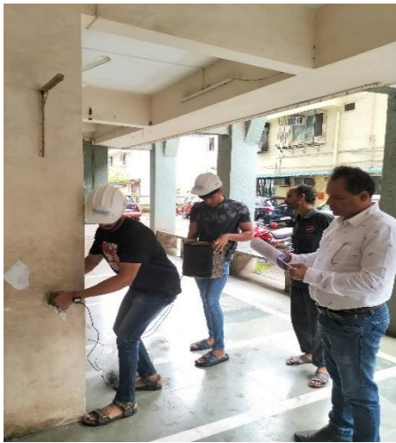
Ultrasonic Pulse Velocity Test (UPV)
